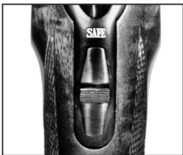
Figure 2. Safety selector in “SAFE” (full rearward) position. The safety selector should be in this position when the under-lever is open to load a cartridge, or to unload a live round. Whenever a cartridge is chambered, the safety selector should be in the “SAFE” position unless the rifle is to be fired immediately. Keep the safety in this position except when actually firing. (When the safety is in the “SAFE” position, it is referred to as being “on.”)
