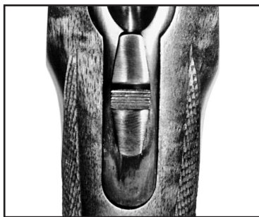
Figure 3. Safety selector in “FIRE” (full forward) position. The safety selector should be moved to this position only when the gun user is actually firing the rifle. If you chose not to fire, immediately return the safety to the “SAFE” position shown in Figure 2. When the safety is in the “FIRE” position, it is referred to as being “off.”
