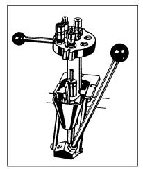
and position it against the edge of your bench top in the most convenient location, usually near the center of the bench, leaving a work area on each side of the press. Mark the position of the mounting holes and drill them; then, using ¾" bolts and suitable washers and nuts, securely anchor the press.
