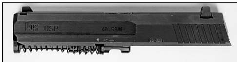
Figure 32B (recoil/buffer spring assembly and barrel locking block properly positioned in the slide)
