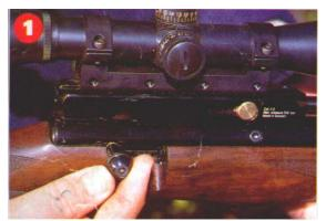
Draw back cocking bolt fully and push sliding magazine to right-hand side.
