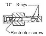
Before inserting into the rifle, the probes "O"- Rings should be carefully examined (if any damage is evident the "O"- Ring must be changed before continuing), and ensure a small amount of molycote 111 grease is applied to "O"- Rings The quick fill device is fitted on the front of the air cylinder. Unscrew the endcap, turning anticlockwise to reveal the quickfill inlet.
