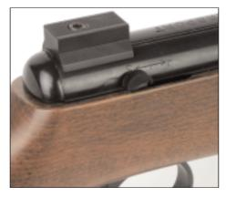
advised that you also fit a BSA scope stop kit (part no. 18-1178) which has a shock absorbing pad to help protect the scope from recoil action. Single screw mounts should not be used.
